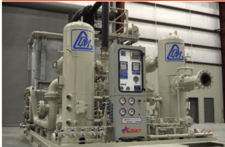
■ This new Alegacy Caterpillar G3408TA engine-driven Ariel JGJ/2 reciprocating compressor package is shown ready for shipment to CDM Resource Management.
